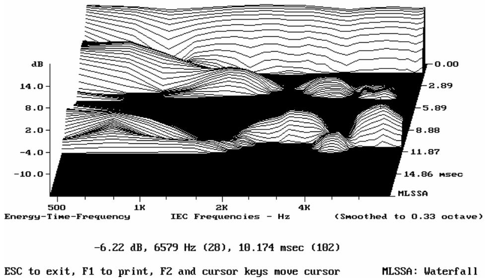
Fig. 13. Time-frequency response, Centre-Front loudspeaker, initial construction.
