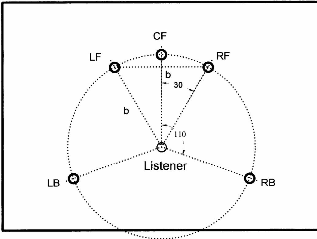
Fig. 5. Loudspeaker layout for five-channel multichannel sound from Ref. 2.
