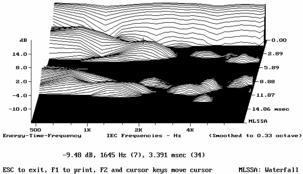
Fig. 10. Time-frequency response, Left-Front loudspeaker, initial construction.
