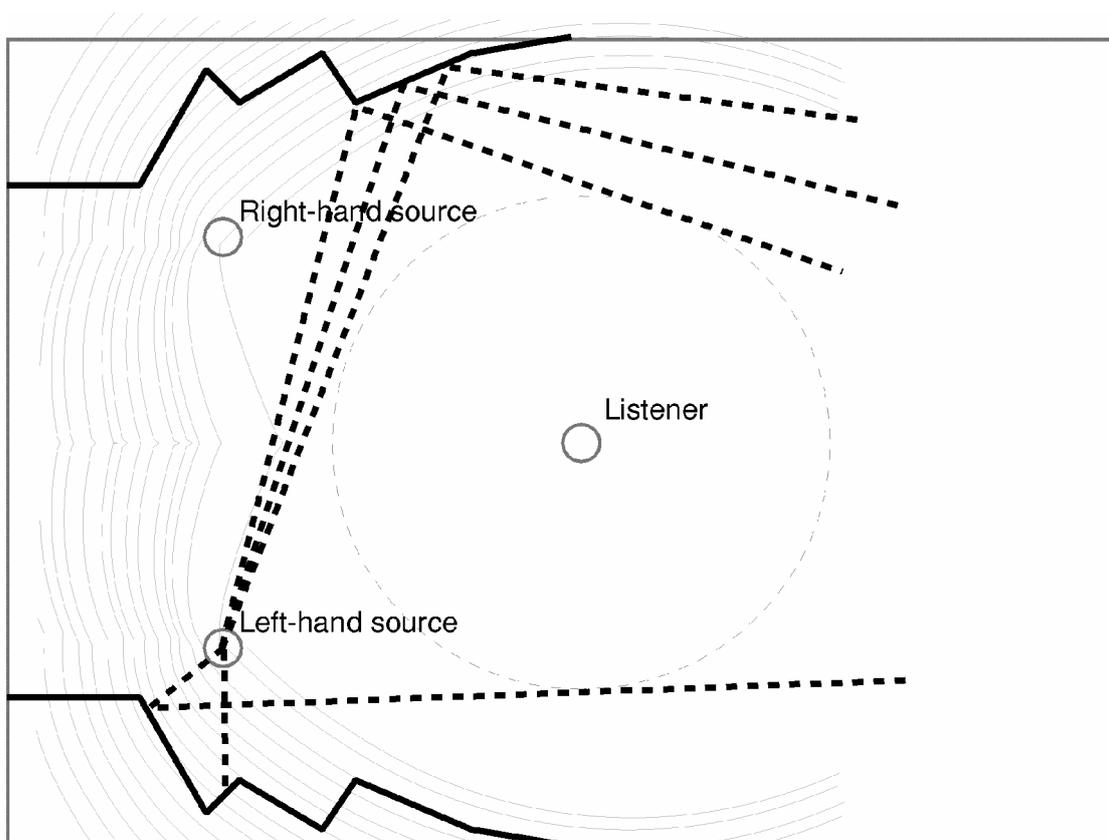
Figure 2. Room layout for reflection control with flats and reflections.
