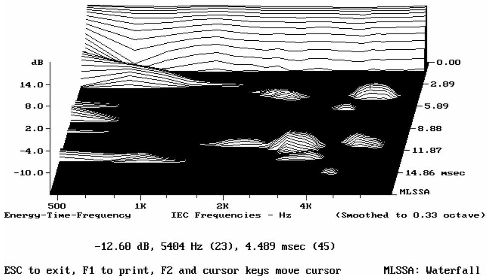
Fig. 14. Time-frequency response, Centre-Front loudspeaker, after replacement of rear wall diffusers and with floor reflector
